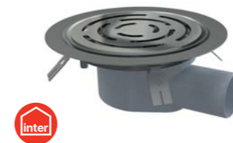
APV3513 Floor drain 105x105/50 mm side outlet, stainless steel grid, stainless steel flange and collar-2nd level insulation, combined odour trap SMART
